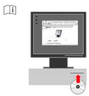
6. To optimize your monitor image, press the Automatic Image Setup key. Automatic image setup requires that the monitor is warmed up for at least 15 minutes. This is not required for normal operation.
